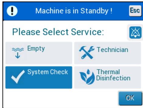
Figure 42: Selecting System Check
