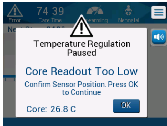
Figure 40: Controlled Rewarming Mode: Core Readout Too Low Message
