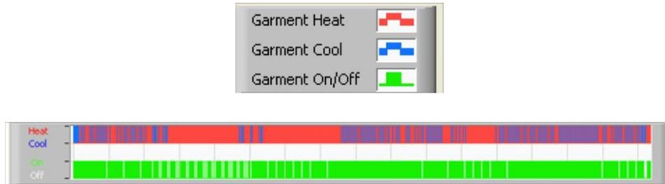
**Heat/Cool-** When CritiCool® is cooling the water in the tank, the line is blue. When the device is warming the water in the tank, the line is red.
