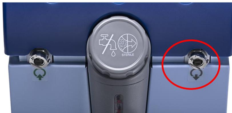
To resolve, press “Esc” on the screen. Keeping track of which tube was where, disconnect each connecting water tube at the machine end, then reconnect in the reverse way. Now the male draining connector should be connected to the tube inserted into Water Out. When done, follow the prior steps once more to continue emptying.
