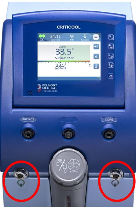
There are two Quick Coupling Connectors below the Core and Surface Temperature Probe Sockets:
