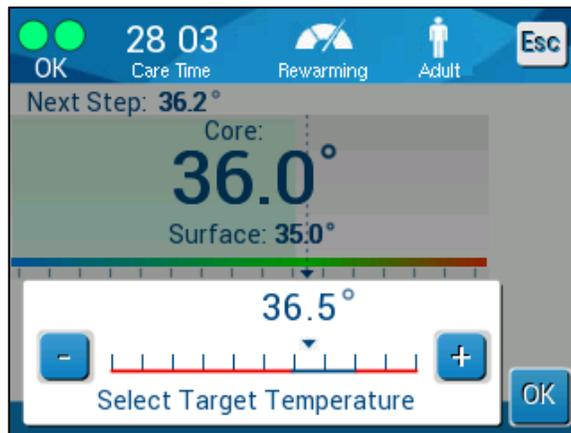
**Figure 30: Target Temperature Setting Panel**
