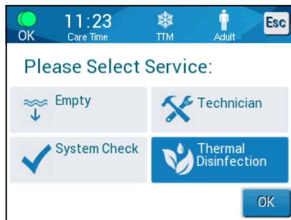
The thermal disinfection of CritiCool® is an integrated feature, which heats the circulating water of the system, thus allowing the heat to disinfect the internal water pathways of the system, including the water tank.
