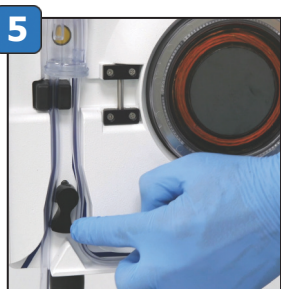
Place the infuse line to the left of the valve wand and the thinner recirc line to the right of the valve wand
