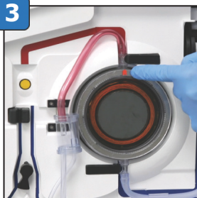
Load the circular heat exchanger with the red arrow pointing up
