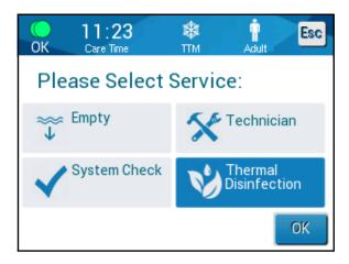
The thermal disinfection of CritiCool<sup>®</sup> is an integrated feature, which heats the circulating water of the system, thus allowing the heat to disinfect the internal water pathways of the system, including the water tank.
