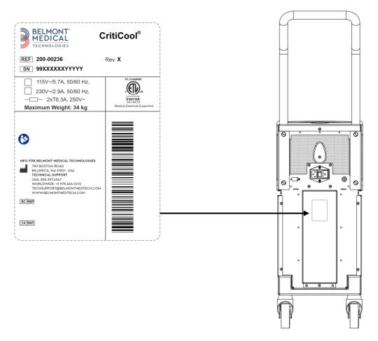
Figure 1: Label Placement for the CritiCool® Device.
