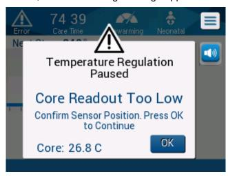
Figure 40: Controlled Rewarming Mode: Core Readout Too Low Message.
