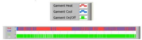
**Heat/Cool-** When CritiCool® is cooling the water in the tank, the line is blue. When the device is warming the water in the tank, the line is red.
