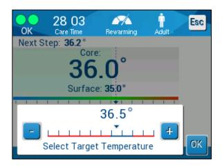
Figure 30: Target Temperature Setting Panel
