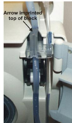
3. Firmly position the interlock block into the fluid out detector.
