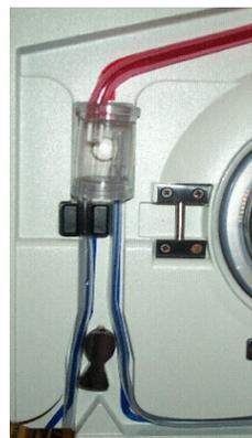
5. Place the pressure chamber into the pressure chamber well. Firmly insert the wider infuse line into the air detector and to the left of valve wand.
