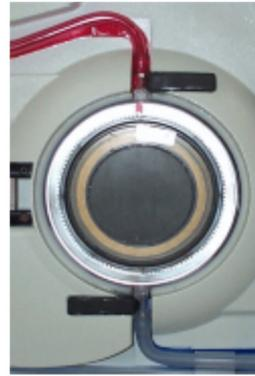
1. Snap reservoir chamber into the reservoir support clamp.
