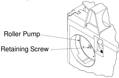
The pump head can be removed and cleaned if needed.
