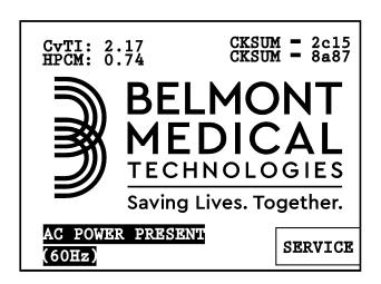
Pressing the SERVICE key accesses the SERVICE mode. This key appears on The Belmont logo screen only at system powered-up. This screen remains active for 4.5 seconds before the system enters the PRIME mode.
