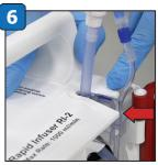
Firmly position the interlock block on top of the shelf with thinner recirc line to the right the blue arrow pointing inward
