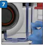
Place the larger blue tubing in the groove to the left and the smaller tubing to the right, close and latch the door
