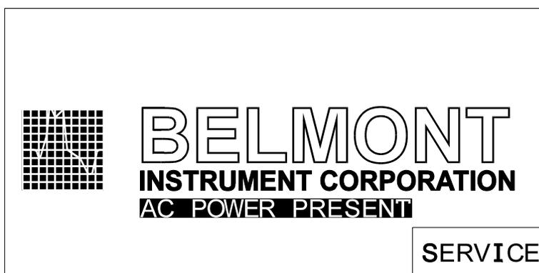
Pressing the SERVICE key accesses the Calibration/Set-up mode. This key appears on the BELMONT logo screen only at system powered-up. This screen remains active for 4.5 seconds before the system enters the Prime mode.
